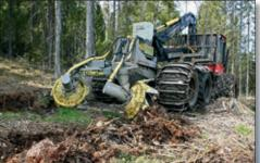
The T21.b mounted on a smaller forwarder
