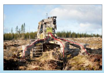
The Bracke \$35.a can be attached to a one-, two-, or three-row scarifier.
