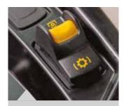
PTO engagement remains electro-hydraulic using the same 3-position safety switch (On, Off and Lock/brake).
